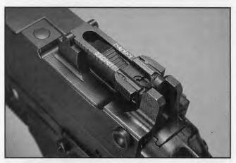
SS-77's folding-leaf rear sight has been taken from the FN MAG 58 and provides a peep aperture in the down position for ranges from 200 to 800 meters.
